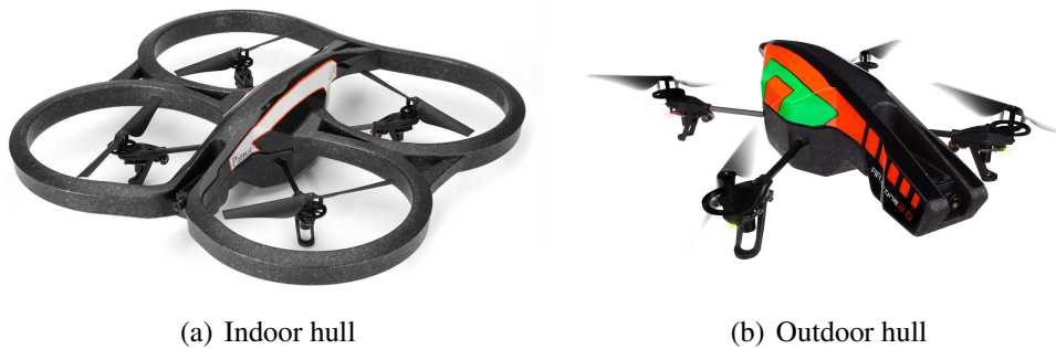
Figure 2.2: AR.Drone 2.0 and its different hull options
