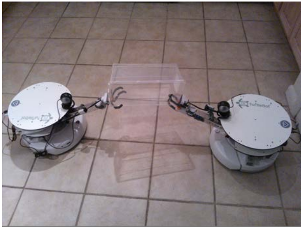
Fig. 1. Two robots cooperate to lift an object under the direction of the human operator. In the multi-robot manipulation task, the robots must lift and deliver a series of objects of different sizes to the goal location.
