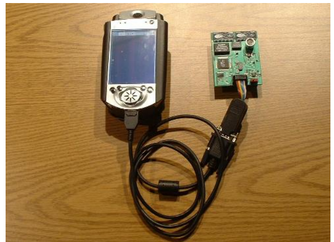
Figure 1: Each participant in the CTF game is equipped with the hardware shown above. Left: the iPAQ H3650 handheld and BackPAQ interface sleeve. The BackPAQ provides several I/O options including an accelerometer, camera and 802.11 wireless communication. Right: the Cricket listener (indoor location sensor) provides an estimate of the user's global position.
