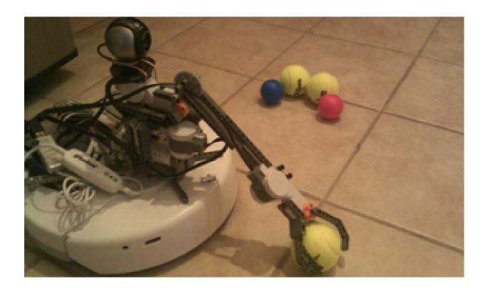
Figure 6: HU-IE combines a mobile base (3 DOF) with a robot arm (2 DOF) equipped with a gripper. This enables HU-IE to navigate indoor environments and pick up small objects. The user can wirelessly teleoperate the robot using a webcam.
