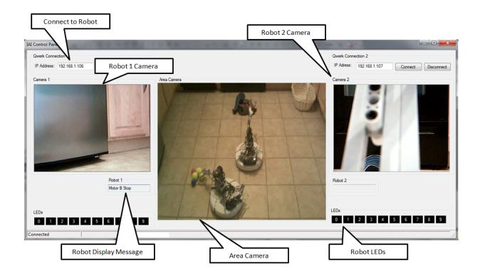
Figure 31: The user interface is designed to enable the user to seamlessly switch teleoperation between multiple robots. The IAI supports a cooperative mode where the agent supports the user's active robot by mirroring its planned actions. The user views the environment through an overhead camera and the robots' webcams.
