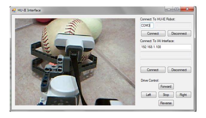
Figure 8: The user views the object being manipulated through a webcam mounted on the robot's arm.
