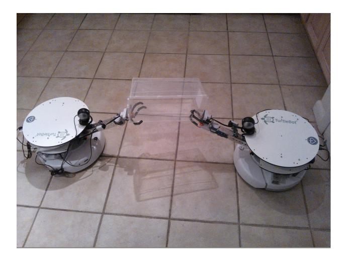
Figure 9: Two robots cooperate to lift an object under the direction of the human operator. In the multi-robot manipulation task, the robots must lift and deliver a series of objects of different sizes to the goal location.
