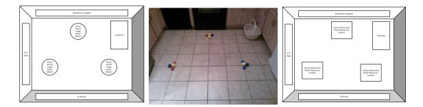
Figure 50: The two robots operate within a  $6.3' \times 6.4'$  household area and move objects from various piles to the goal area. Scenario 1 (left, middle) contains piles of small objects that can be moved with a single robot, whereas Scenario 2 (right) contains objects that require bimanual manipulation.
