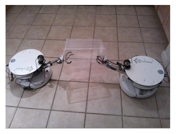
Figure 47: Two robots cooperate to lift an object under the direction of the human operator. In the multi-robot manipulation task, the robots must lift and deliver a series of objects of different sizes to the goal location.
