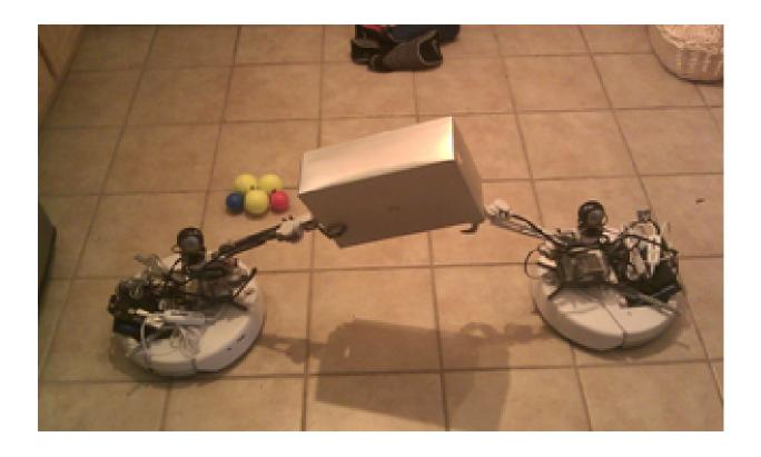
Figure 23: Two HU-IE robots cooperate to lift an object. One robot is teleoperated while the other moves autonomously to mirror the user's intentions. The user can seamlessly switch robots during such maneuvers.
